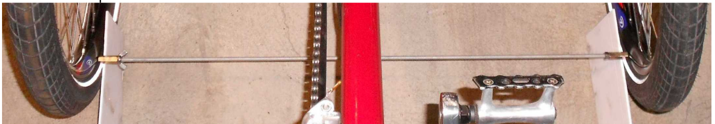
Fig. 1 Set-up with simple adjustable rod toe-in measuring aid and equal height rests.
