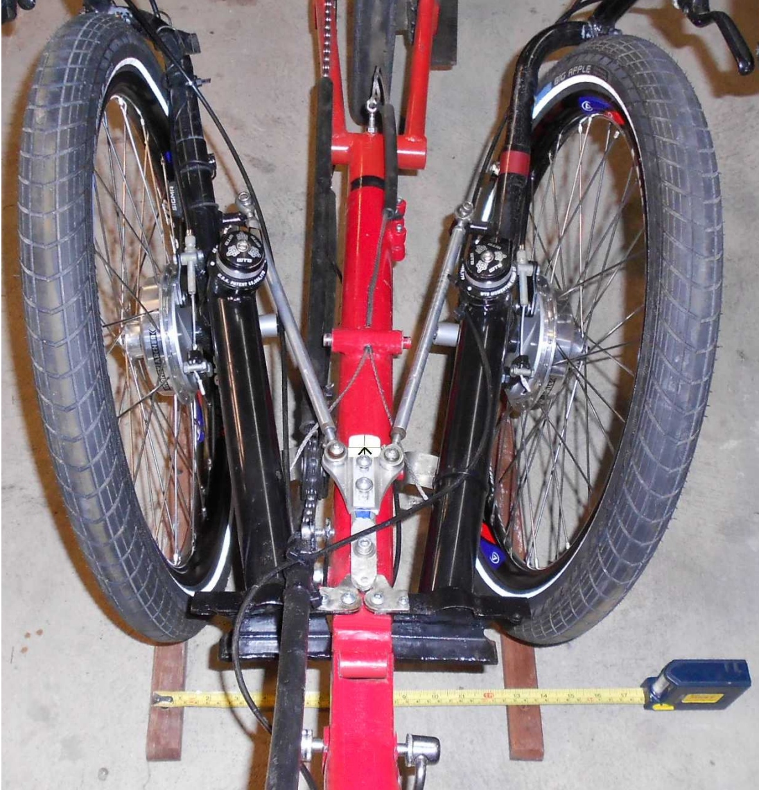
Fig.3 Folded wheel toe-in setup
